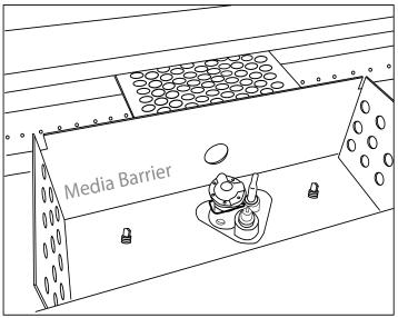
Fig. 6 Show pilot assembly under the pilot hood.
