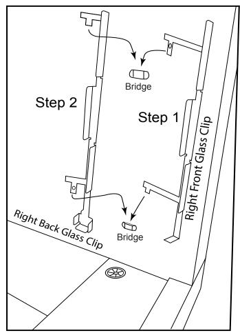
Fig. 20 Installing glass clips.
