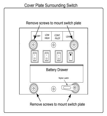
Mounting plate under switch cover LOW CONT. ON/OFF LEARN PILOT (4) 0 0 0 5 <sup>5</sup>/<sub>8</sub>" **Battery Drawer** (<del>}</del>) 0 0 0
