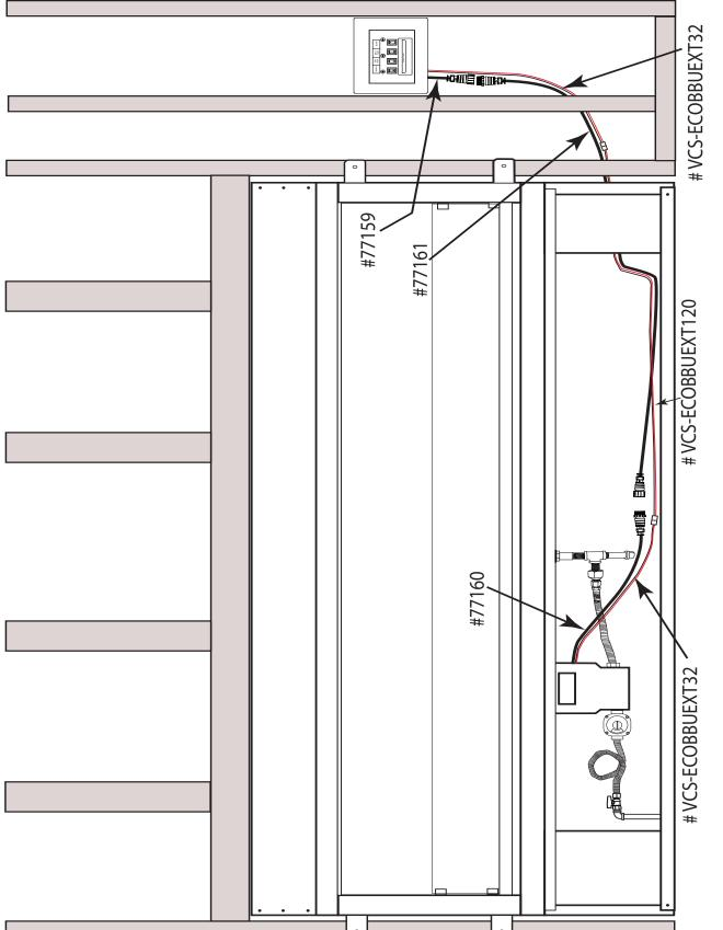
Fig. 13 Overview of fireplace wiring to control box. Note: The fireplace is provided with 10-feet of wire. If you require a longer length, an optional 10-foot wire harness 77161 & VCS-ECOBBUEXT120 are available in replaemet parts section.
