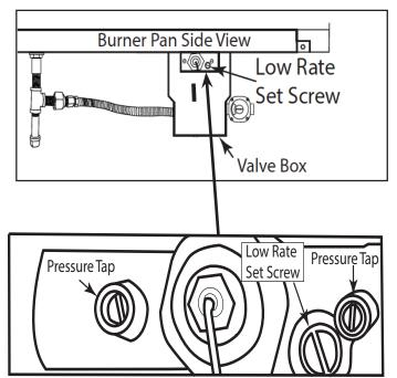
Fig. 10 Detailed location of low rate set screw
