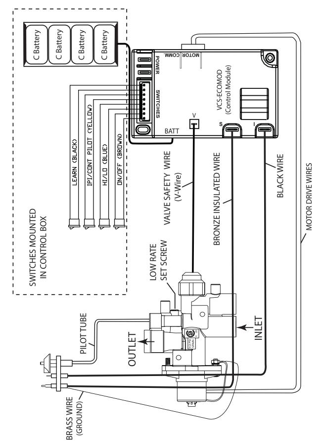
Fig. 19 This wiring diagram shows the components inside the valve box. The dotted line box shows the components external of the valve box.
