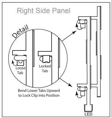
Fig. 21 Detail close up of glass clips.
