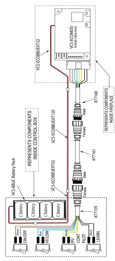
Fig. 18 This wiring diagram shows wiring from control panel and battery pack to control module. Each is independent of the other.
