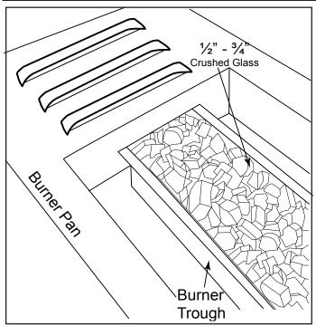
Fig. 29 Installing media.
