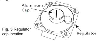
**Step 5:** On the underneath side of the aluminum cap is a plastic stem. Using a 6mm wrench remove the stem, unscrew the stem (counter-clockwise), turn it over and install the opposite end back into the cap. See Fig. 4.
