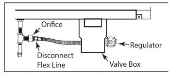
Fig. 2 Changing main burner orifice
