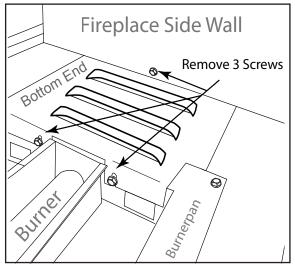
Fig. 2 Removal of burner pan screws.
