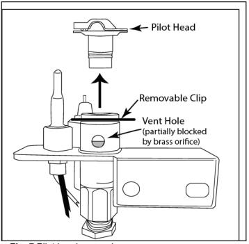
Fig. 7 Pilot hood removal
