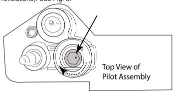
Fig. 8 Shows slot inside pilot orifice
