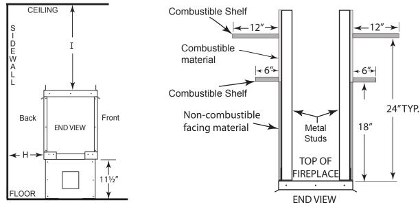
**Fig. 10** See-through fireplace clearance to combustibles (See Table 6)
