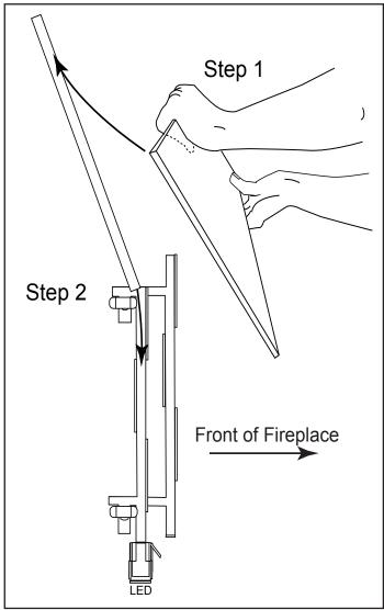
Fig. 34 Installing windshield into clips (glass holders).
