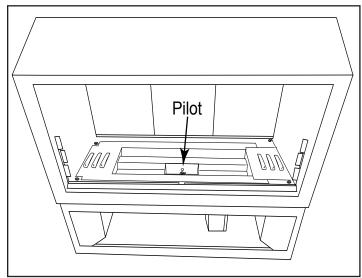
Fig. 24 Shows burner pan installed into fireplace.
