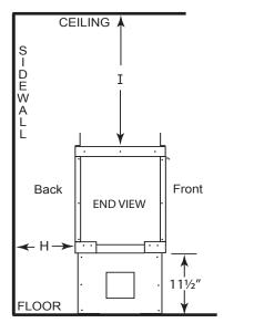
**Fig. 6** Single-sided fireplace clearance to combustibles (See Table 3)
