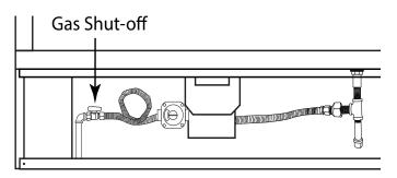
**Fig.1** Close up view of inlet gas connection with shut-off valve.
