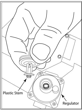
Fig. 5 Regulator stem shown in LP setting
