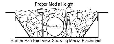
Fig. 30 End view of burner with media.
