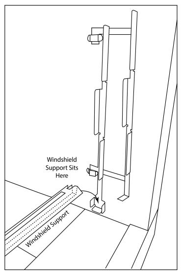
Fig. 23 Installing windshield support.
