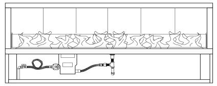
Fig. 35 Proper flame height.
