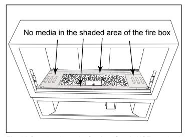
**Fig. 31** Covering the entire fireplace floor is NOT permitted in the shaded area.
