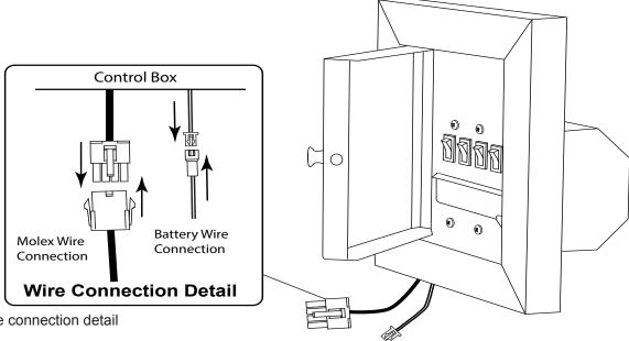
Fig. 16 Wire connection detail
