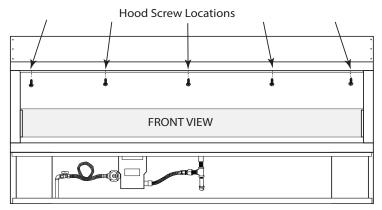
Fig. 32 Installing hood(s) on the fireplace.
