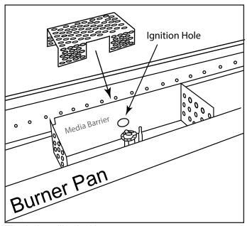
Fig. 25 Installing ignition screen.
