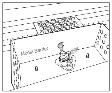
Fig. 28 Proper pilot flame through ignition hole.
