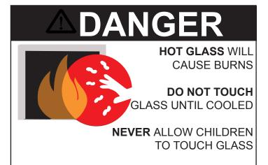
A barrier designed to reduce the risk of burns from the hot viewing glass is provided with this appliance and shall be installed for the protection of children and other at-risk individuals.
