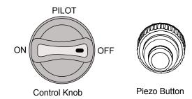
Fig. 11 Control panel with gas valve knob and Piezo.
