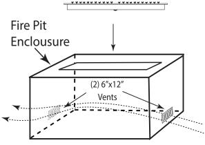
Cross Flow Ventilation (Min. 18 Sq. In. Per Side) Fig. 3 Cross ventilation example
