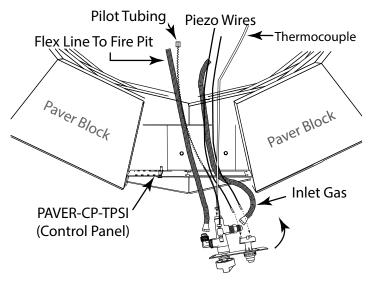
**Fig. 6** Installing control panel into PAVER-CP-MT mounting plate.
