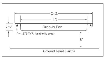
Fig. 1 Burner pan specifications.
