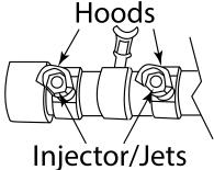
Fig. 9 Correct placement of injector hoods.
