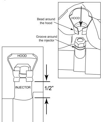
Fig. 9 Installing injector hoods.
