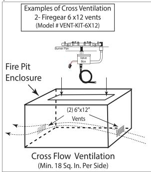
Fig. 3 Shows cross ventilation for a linear enclosure.
