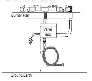
Fig. 1 Flat burner pan specifications.
