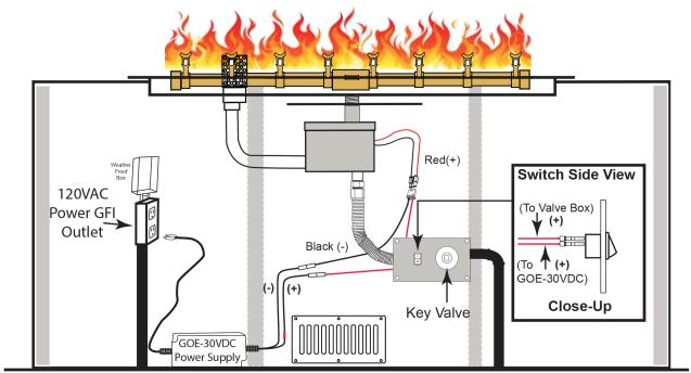
Fig. 5 Show typical wiring diagram with switch.
