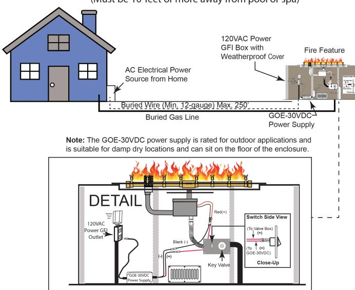
**Fig. 4** Example of a single fire feature install with power supply and switch contained within the enclosure, when applicable.
