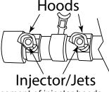
Fig. 10 Correct placement of injector hoods.
