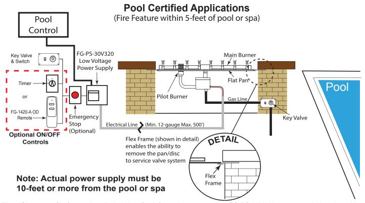
**Fig. 6** Shows any fire feature installed within 5 feet of a pool or spa requires FG-PS-30V320 power supply (purchased separately). **DO NOT USE THE GOE-30VDC. FG-PS-30V320 power supply can be installed up to a maximum of 500-feet away from fire pit.**
