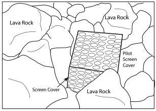
Fig. 11 Media placement around pilot hood.
