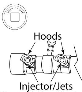
Fig. 7 Proper hood orientation over injectors/jets.
