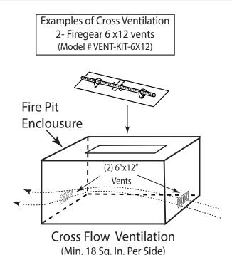
Fig. 4 Cross ventilation example
