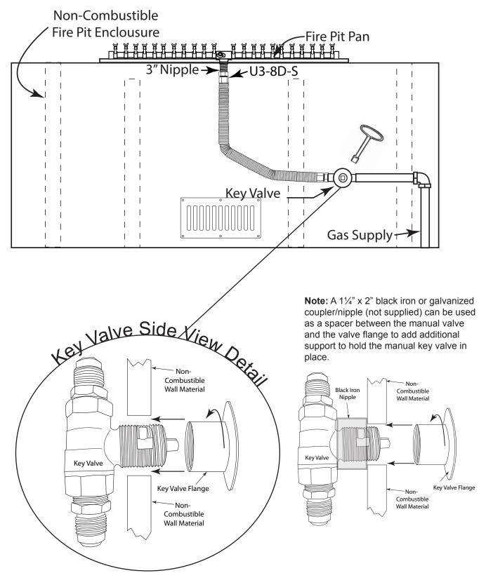
Fig. 7 Typical Installation
