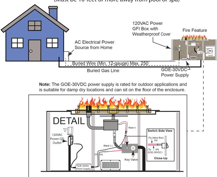
**Fig. 7** Example of a single fire feature install with power supply and switch contained within the enclosure, when applicable. **Note**: Must be 10-feet or more from a pool/spa for this installation. See additional illustration on page 10, Fig. 8.
