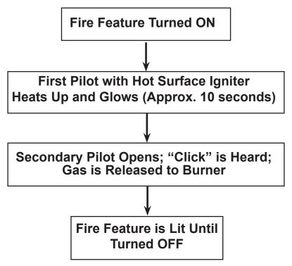
The system is designed to relight itself if blown out. It will try (3) times to relight before it goes into a "hard" lock out.
