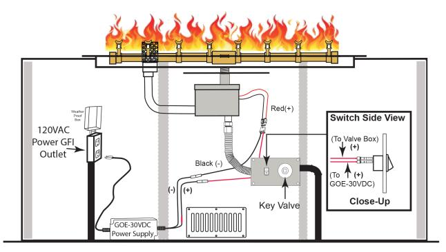
Fig. 8 Show typical wiring diagram with switch.
