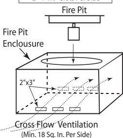
Fig. 3 Shows cross ventilation in a enclosure.
