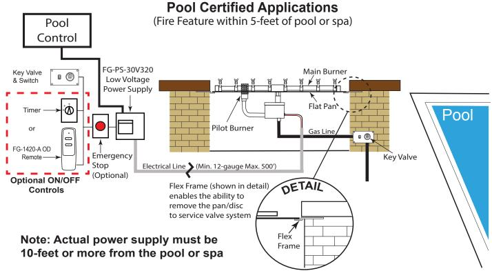
**Fig. 9** Shows any fire feature installed within 5 feet of a pool or spa requires FG-PS-30V320 power supply (purchased separately). **DO NOT USE THE GOE-30VDC. FG-PS-30V320 power supply can be installed up to a maximum of 500-feet away from fire pit.**
