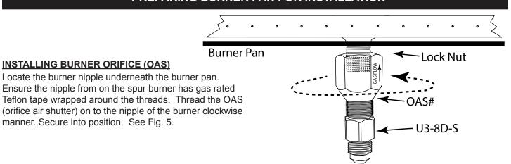
Fig. 5 Installling OAS (orifice) to burner tube.
