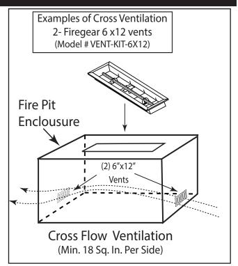
Fig. 4 Cross ventilation example
