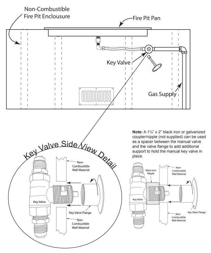
Fig. 7 Typical Installation
