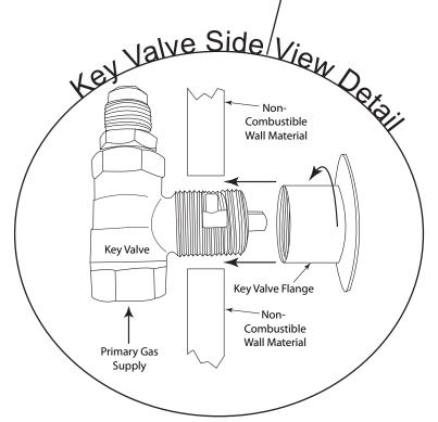
**Note:** A 1½" x 2" black iron or galvanized coupler/nipple (not supplied) can be used as a spacer between the manual valve and the valve flange to add additional support to hold the manual key valve in place.
