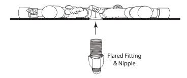
Fig. 4 Installing nipple into bottom of burner.
