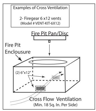
Fig. 5 Cross Ventilation Example
