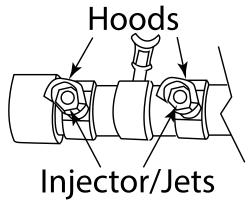
Fig. 9 Proper hood orientation over injectors/jets.
