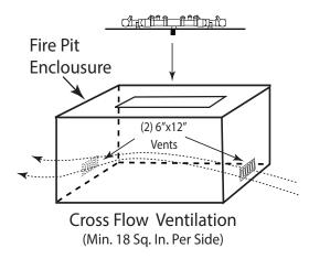
Fig. 2 Cross Ventilation Example
