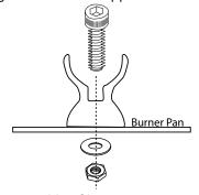
Fig. 7 Shows assembly of burner support to pan.
