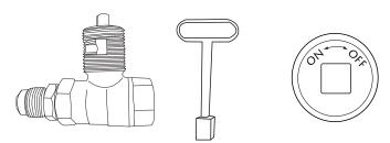
Fig. 10 Key valve components.
