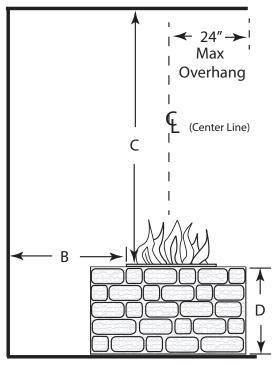
**Fig. 1** Clearance to Combustibles for Table 1 (Not to be used in an enclosed space)
