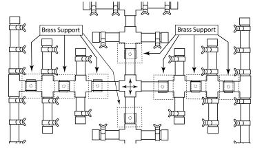
Fig. 6 Locating brass burner supports.
