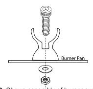
**Fig. 10** Shows assembly of burner support to pan.
