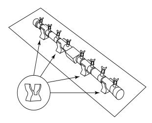
Fig. 11 Shows assembly of burner into pan.
