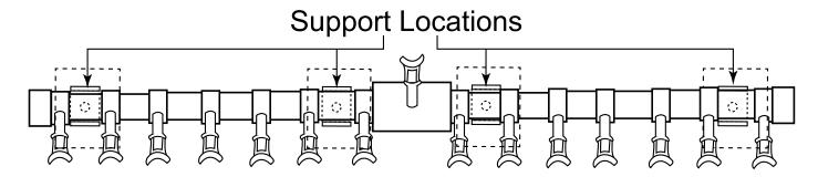
Fig. 7 Locating brass burner supports.
