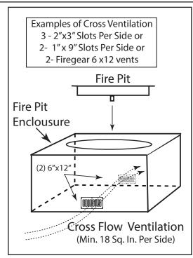
Fig. 3 Cross Ventilation Example
