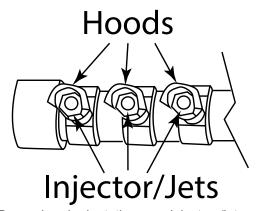
Fig. 8 Proper hood orientation over injectors/jets.
