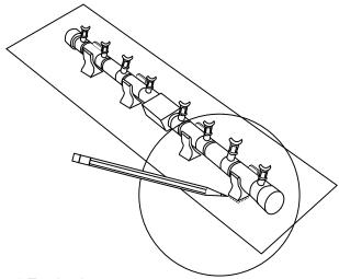
Fig. 9 Tracing burner supports.
