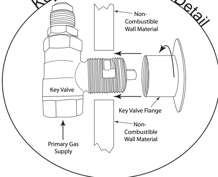
**Note:** A 1 1/4" x 2" black iron or galvanized coupler/nipple (not supplied) can be used as a spacer between the manual valve and the valve flange to add additional support to hold the manual key valve in place.
