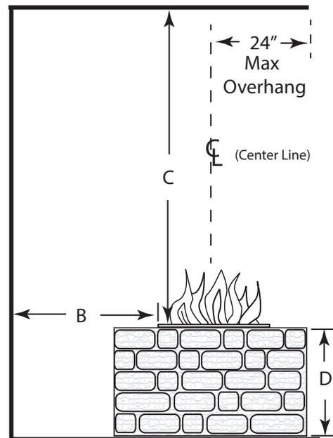
**Fig. 2** Clearance to Combustibles
