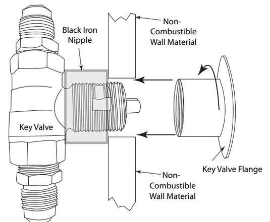
**Fig. 13** Typical installation.
