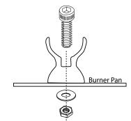
Fig. 9 Shows assembly of burner support to pan.
