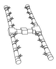
Fig. 5 Shows burner with nipple installed.
