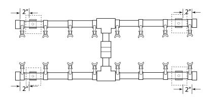
Fig. 7 Locating brass burner supports.
