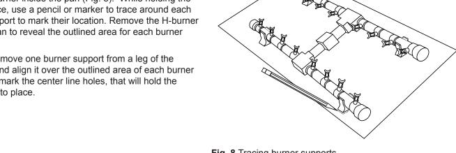
Fig. 8 Tracing burner supports.
