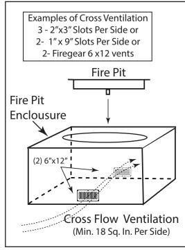
Fig. 3 Cross Ventilation Example
