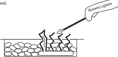
Fig. 15 Lighting fire pit with lighter
