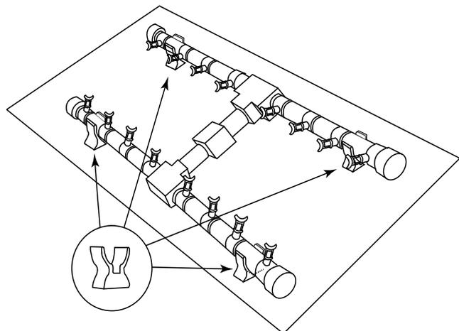
**Fig. 10** Shows assembly of burner into pan.
