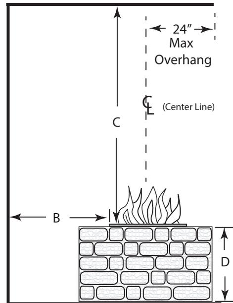
**Fig. 2** Clearance to Combustibles
