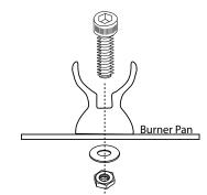
Fig. 9 Shows assembly of burner support to pan.
