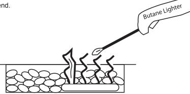
Fig. 15 Lighting fire pit with lighter
