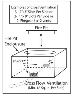
Fig. 3 Cross Ventilation Example
