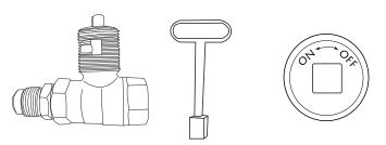
Fig. 11 Key valve components.
