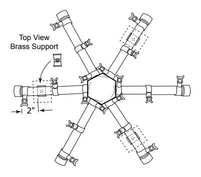
Fig. 7 Locating brass burner supports.
