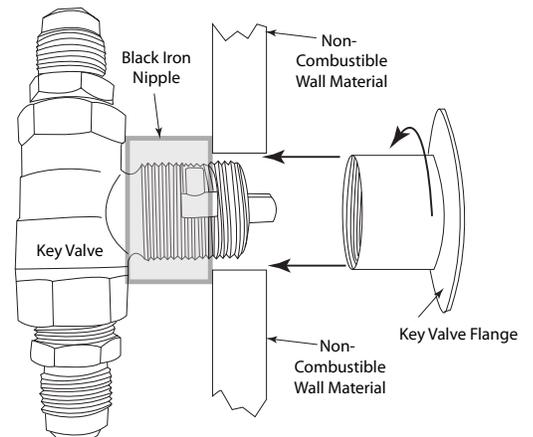
**Fig. 12** Typical installation.
