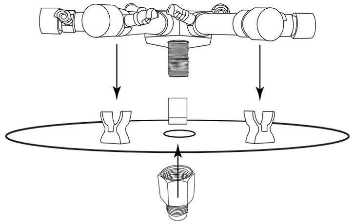
Fig. 10 Shows assembly of burner into pan.
