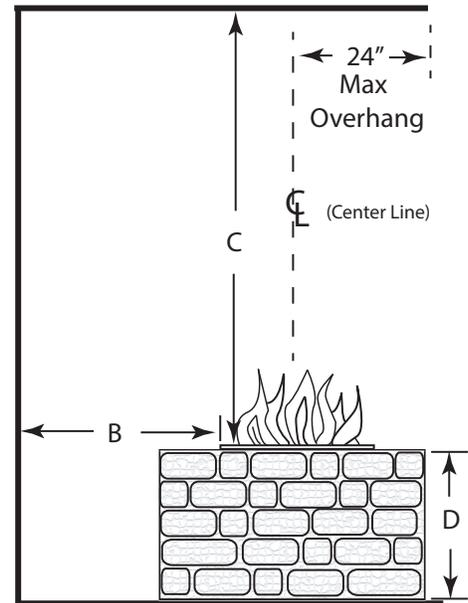
**Fig. 2** Clearance to Combustibles
