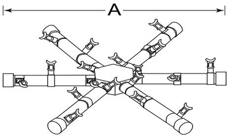
**Fig. 1** Pro Spur Burner Dimensions; refer to Table 1.
