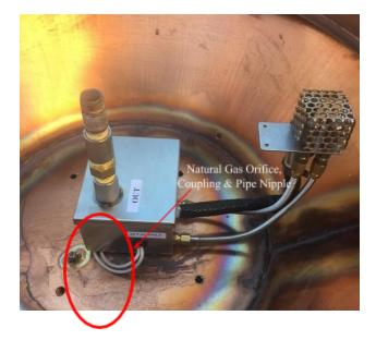
The photo at right shows what the AWEIS looks like just prior to installing the burner pan
