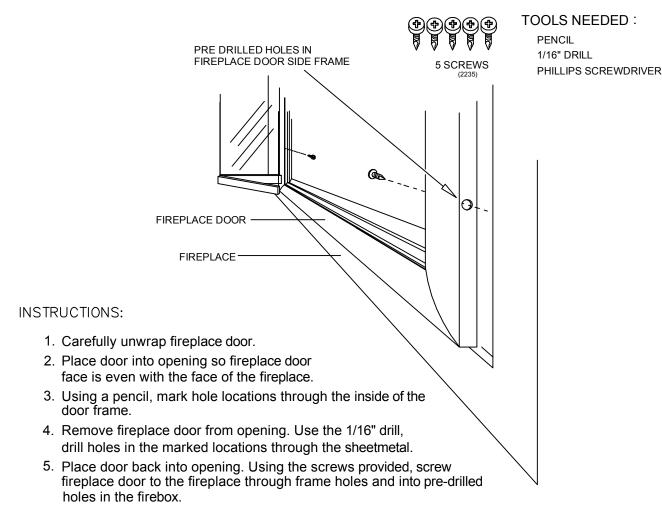
NOTE: self drilling screws are provided to eliminate pre-drilling and speed up the installation. A screwgun with a magnetic tip is required. Care should be taken when using a screwgun to avoid slipping off of the screw and damaging fireplace door.
