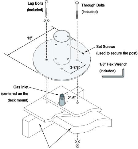
The post mount <u>must be secured to deck framing in four locations</u> (or other secure footing - the deck surface is not adequate for proper support).
