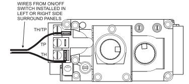
NOTE: TO OPERATE INSERT WITH SIDE PANEL ON/OFF SWITCH, BE SURE TO PLACE THE MAIN SWITCH (TO THE RIGHT SIDE OF GAS VALVE) TO "OFF" POSITION
