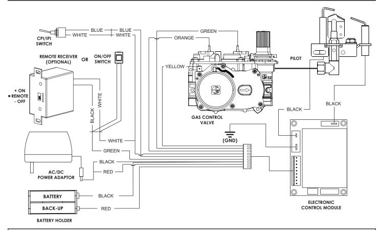
If any of the original wire as supplied with this unit must be replaced, it must be replaced with equivalent gauge and temperature rated wire.
