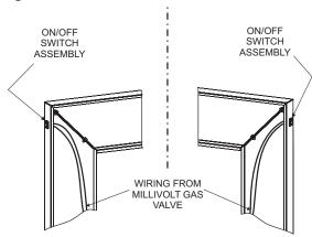
Figure 17 Insert ON/OFF switch into side panel then attach wire assembly from valve terminals.
