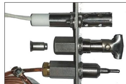
Figure 9.3 – Cleaning pilot orifice
